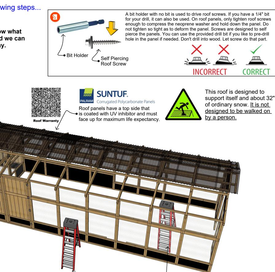
Where to put a screw on a corrugated panel is a topic of debate. Technically, screws can either be installed on the rib tops or in the flats. Where panels overlap it might make the most sense to place on the rib top. Palram, the manufacturer of the panels suggests they be placed on the rib top in all circumstances.
