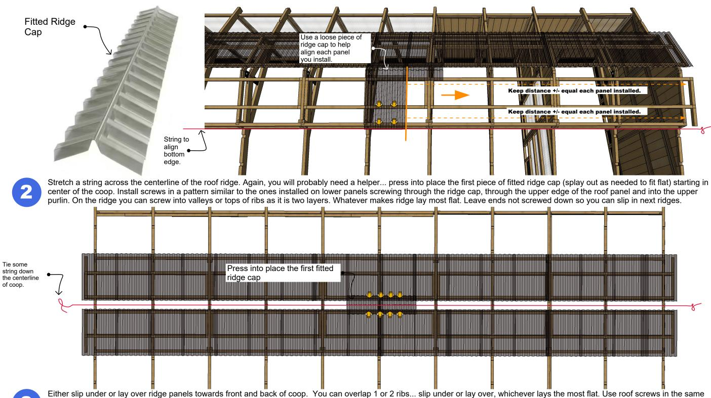
pattern as the roof panels below to attach ridge cap. Extra screws can be used to pin more flat if needed. Extend out even with roof panels on each end or 1 rib extended. Remove centerline string from under ridge when done.
