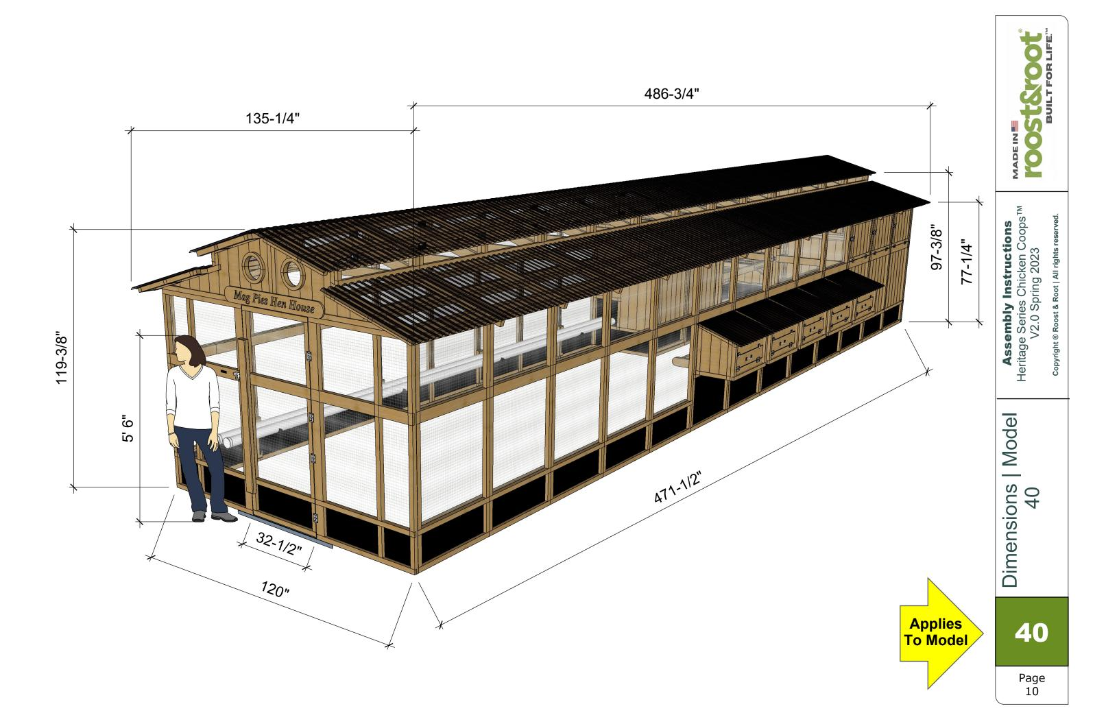
**Note:** If a concrete footer is poured and it is flush with ground level, you can omit pouring footer for interior roost and shed walls. If it is elevated any above ground level, you should pour footer under interior walls too for support. Pouring a concrete footer will simplify leveling and squaring and provide the best way to anchor.
