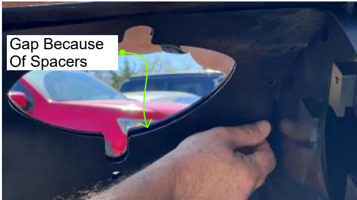
Photo, screwing top edge of liner with spacers between it and back wall... into threaded holes in handle.
