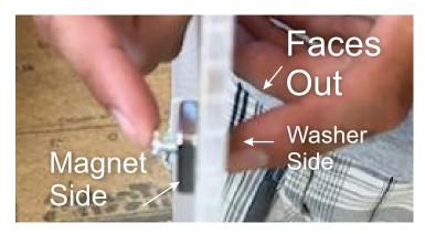
Using a short Chicago screw set, affix the magnet to the <u>same face of the storm panel</u> that washer is on from step 1. Place magnet on one side and metal washer on the other side and hand tighten the Chicago screw set.
